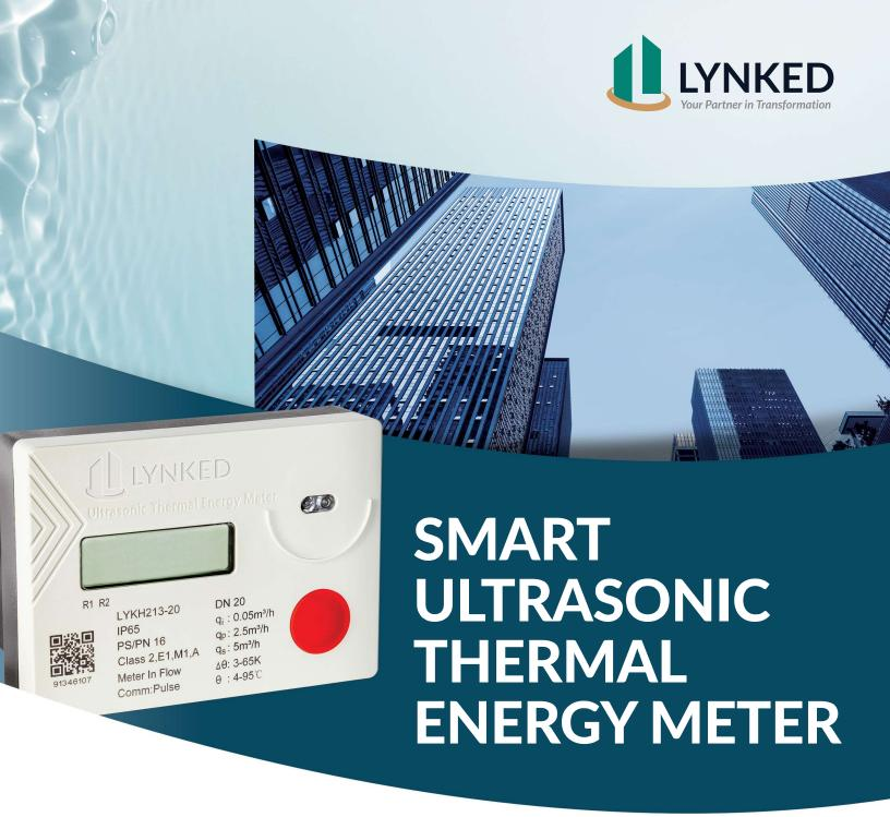
The LYKH series ultrasonic thermal energy meter features a cutting-edge design, with high-quality sensors and instruments to ensure the accurate measurement of heating and cooling energy consumption. The meter has no moving parts, and it uses an innovative time differential measuring principle.
